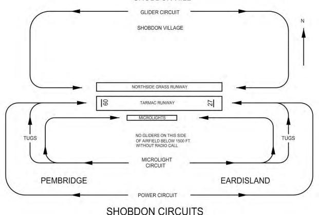
There are 2 new BGA turn points, SH3 and SH4 to the East and West respectively of the airfield. When the task area makes it appropriate, they will be specified to discourage direct, low returns through the power circuit. When required by the task, competitors using them will receive significant bonuses.
